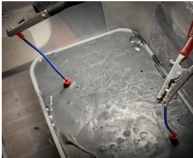
Fig. 1. Electrical resistivity measurement.
